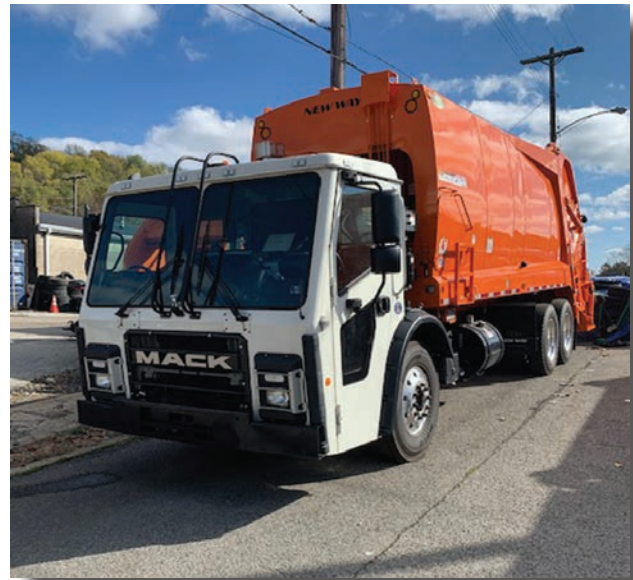
A 2020 New Way 32 LR 64R 25 Yard Rearload Packer. Photo courtesy of the city of McKeesport.
